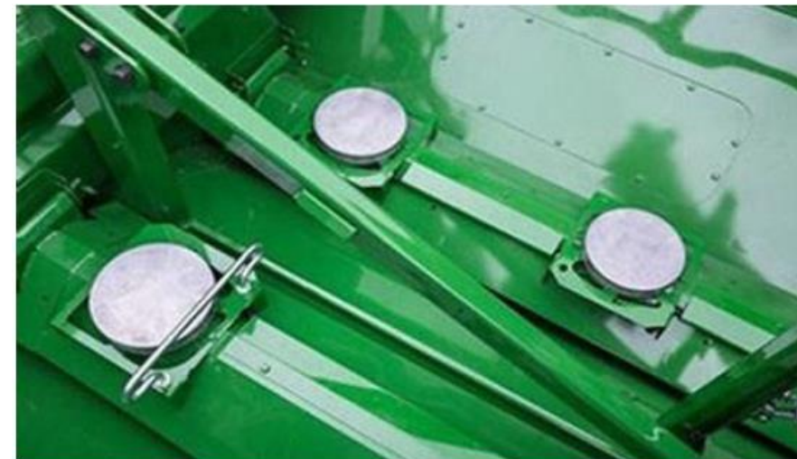
ActiveYield force sensors within the grain tank.
