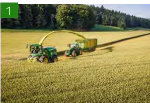
1 Start unloading to the rear (center trailer position)
