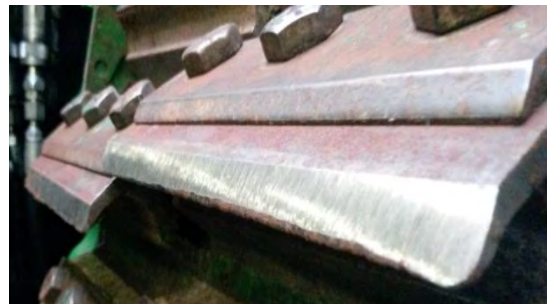
Not enough sharpening
