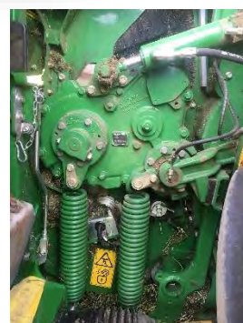
Clean area around feedrolls springs, upper and lower rear feedrolls
