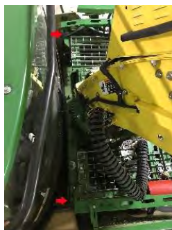
Check area above service compartment behind the Cab
