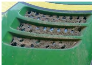
Check the side air inlets on both sides of the machine
