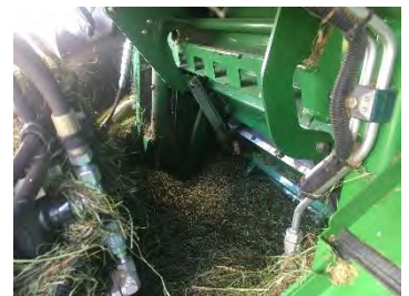
Clean area behind sharpening compartment on top of cutterhead
