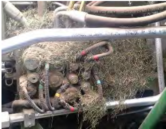
Ensure area around hydraulic valve block is clean
