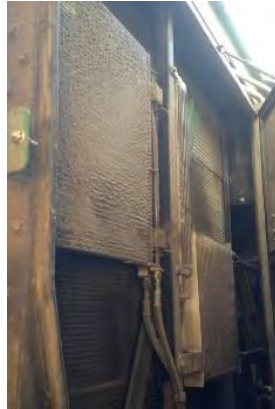
Ensure cooling package is sealed correctly and clean
