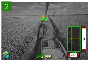
2 If trailer detected, AFC activation possible
