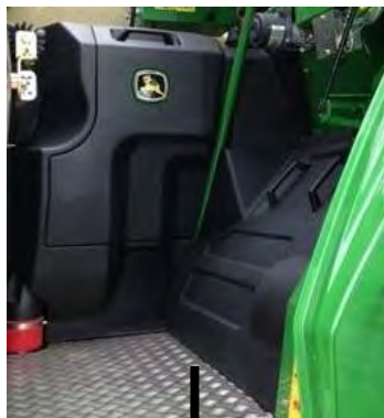
Ensure there is no crop accumulation underneath plastic panels
