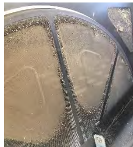
Ensure cooling package is sealed correctly and clean
