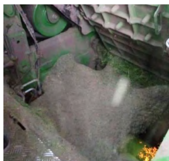
Corn with Kernel Processor in position Grass when Grass Chute in position
