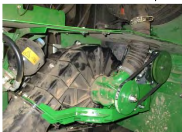
Remove LHS panel periodically to clean this area thoroughly, specifically around Suction Blower Fan.
